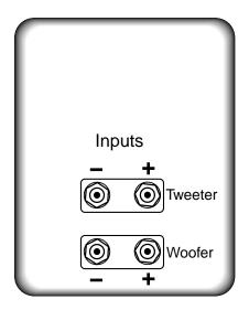
A speaker which can be biamped or biwired will have two sets of binding posts. Sometimes these posts are joined with shorting links for normal operation.
